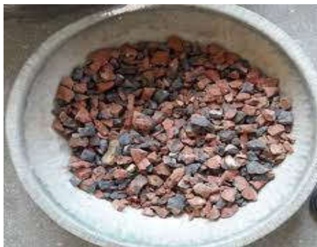
Crushed Zhama Brick
