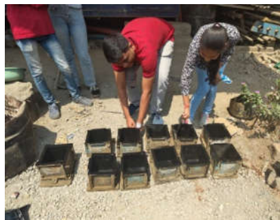
Well finished cubes
