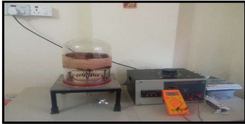
Figure 2- Static gas sensing and Electrical measurement set up
