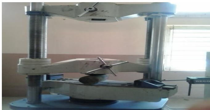
Fig 3.9 Split tensile strength of concrete
