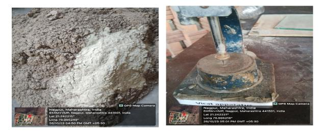
The partial replacement of glass powder according to the IS 4031 part 4 consistency test give the value between 5 to 7 which resulted that Waste Glass Powder and Fly Ash provide the
