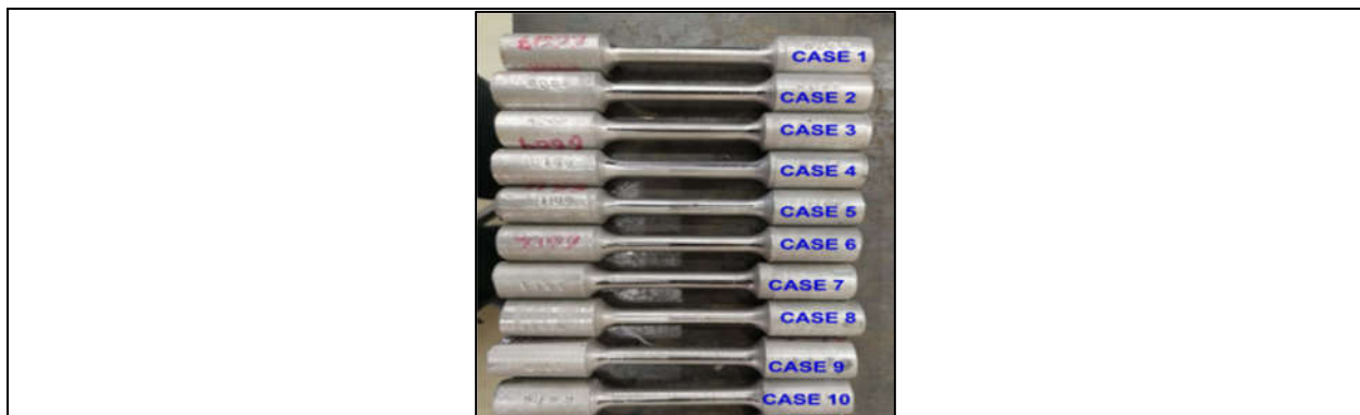
Fig. 9 Test casting samples as per ASTM-B557 for ultimate tensile test
