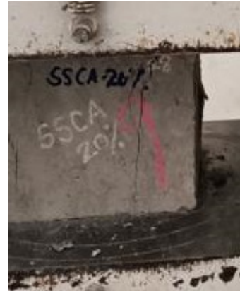
Figure 10. Crack on cubes
