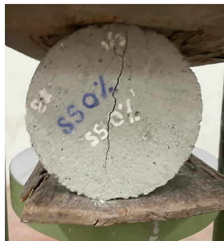
Figure 14. Crack on cylinder
