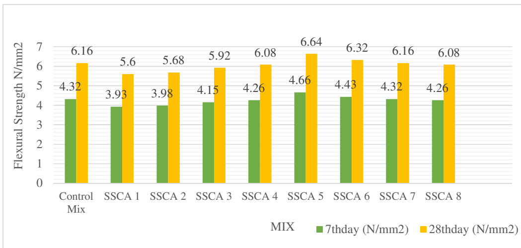
Figure 19. Flexural Strength Graph of Coarse Aggregate Replaced
