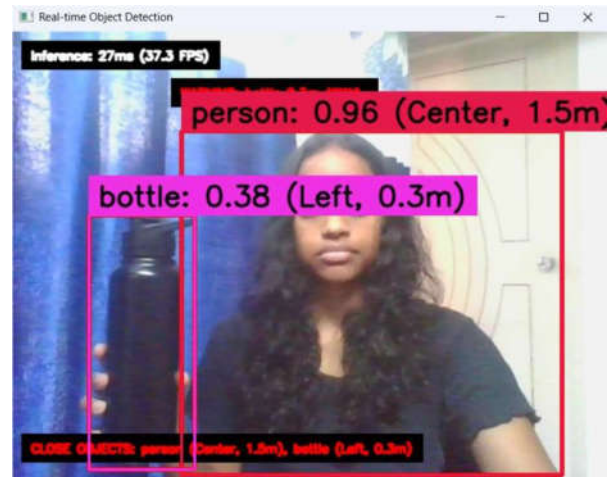
Fig. 5: Real-time Object Detection with Distance and Position Estimation
