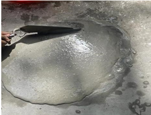
FIGURE 6. Slump Flow of 875mm
