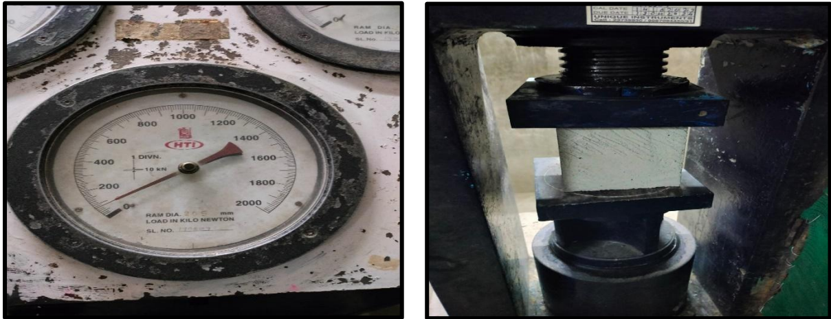
Fig.7. Compressive Strength of AAC Block
