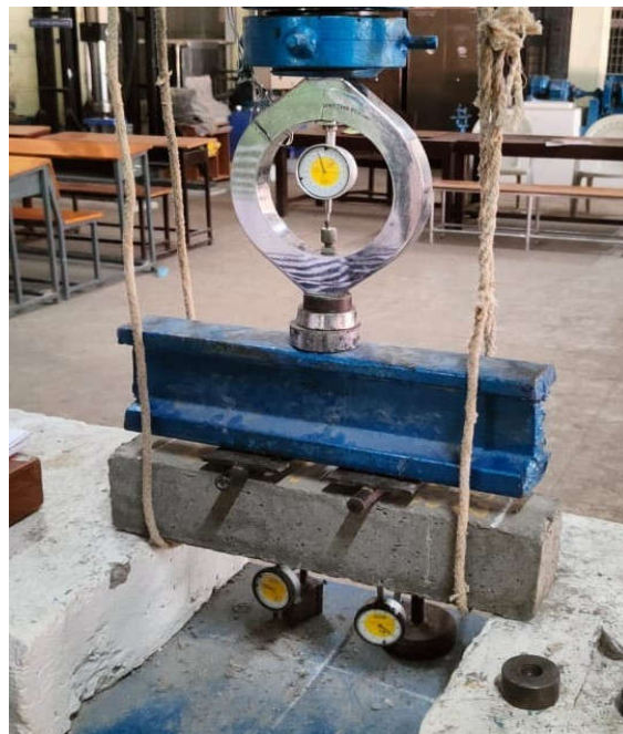
Figure: 5 Beam testing
